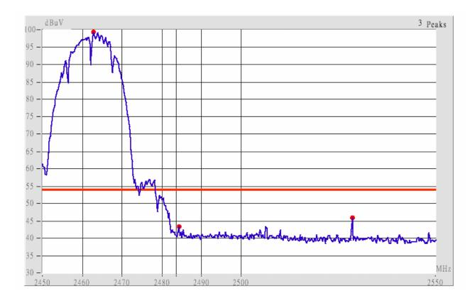
This is the hard copy of our bandedge measurement generated by our bandedge testing program. The picture shown above is the bandedge of channel 11.
