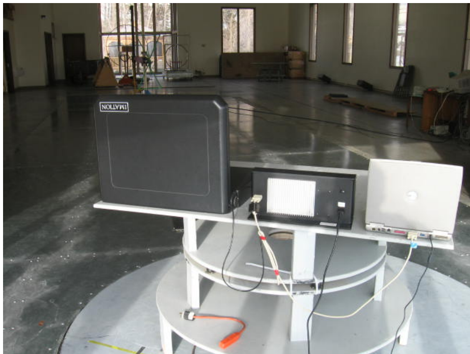
Radiated Emissions Test Configuration
