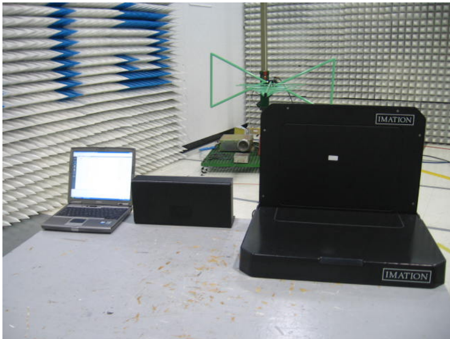
Radiated Emissions Test Configuration
