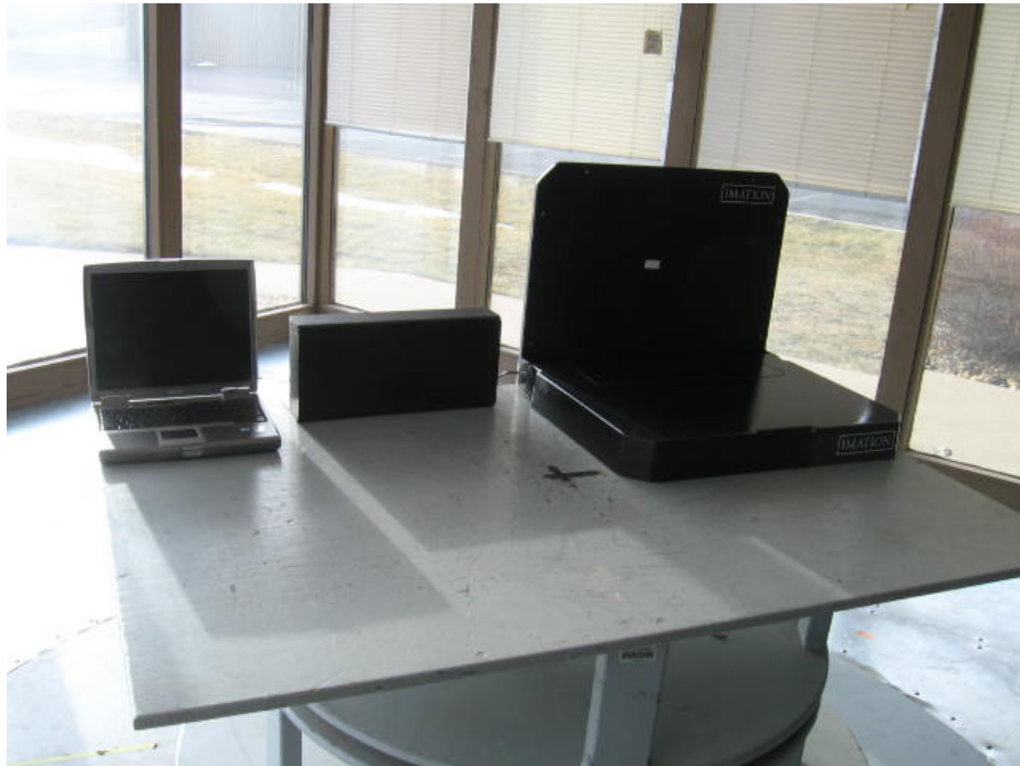
Radiated Emissions Test Configuration
