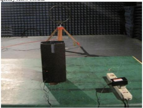
Test frequency from 30MHz to 1GHz for Normal Work mode
