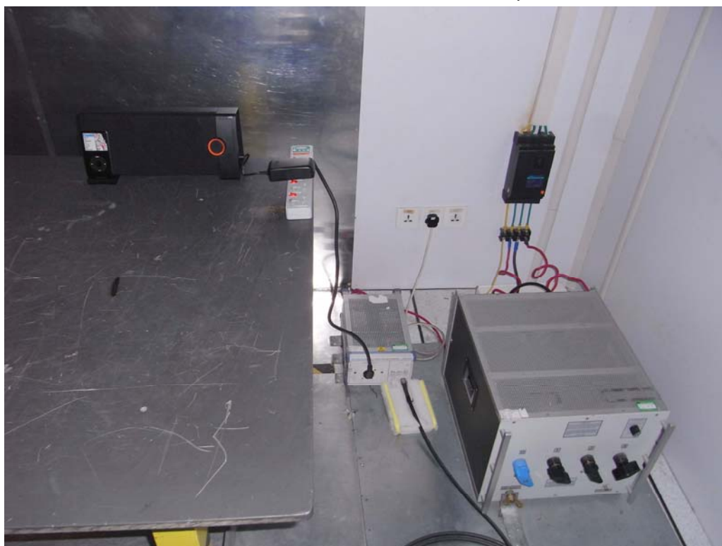
Line Conducted Emission Test Setup
