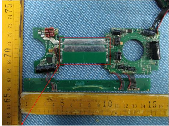
Uses a PCB as the connection, this PCB only used for connection without any electronic components.
