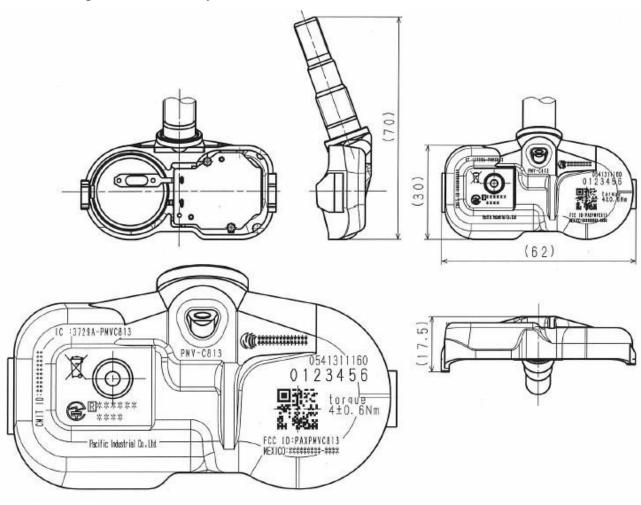
Fig 5. Marking location and dimension
