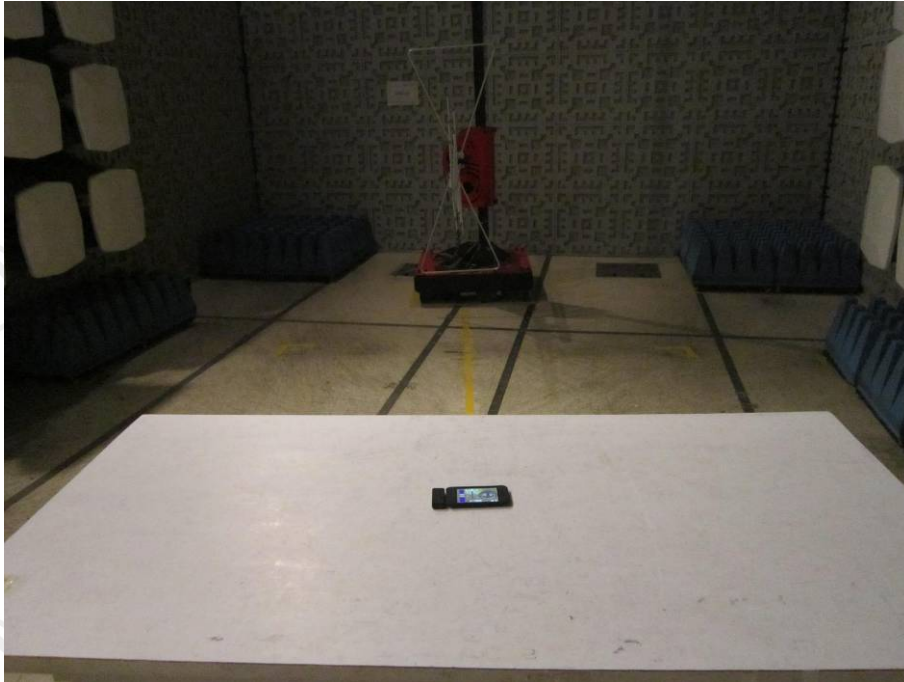
TEST SETUP OF RADIATED EMISSION (30MHz~1GHz)
