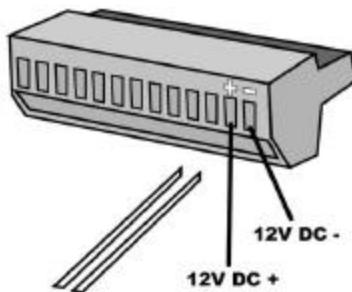
We recommend installing the module using active low momentary switching. Other options are available and a qualified installer should determine the optimal configuration. The attached diagram may be of assistance to a qualified installer.
