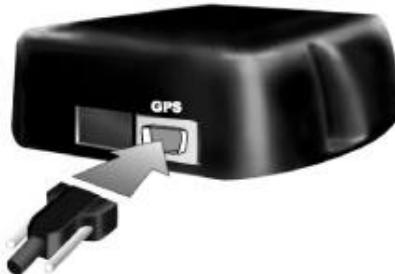
**Note: Plug in the GPS antenna before you connect power to the unit.**
