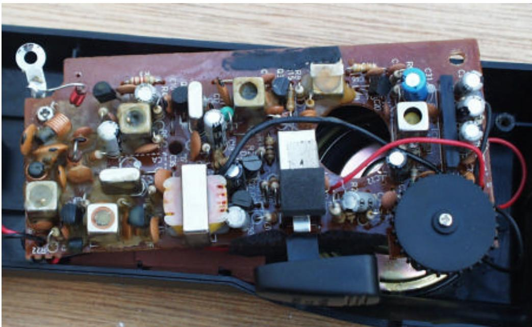
**BOTTOM VIEW OF THE PRINTED WIRING BOARD**
