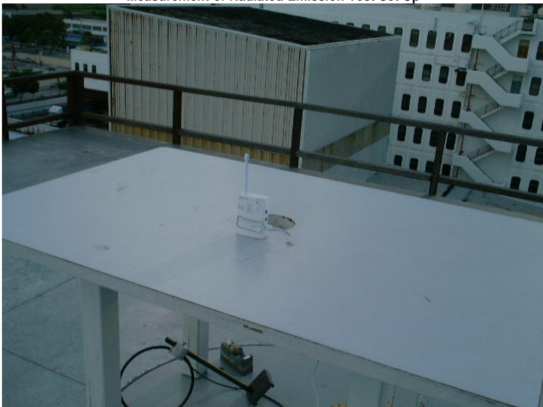
Measurement of Radiated Emission Test Set Up
