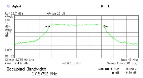
Transmit Freq Error 53.509 kHz x dB Bandwidth 17.713 MHz
