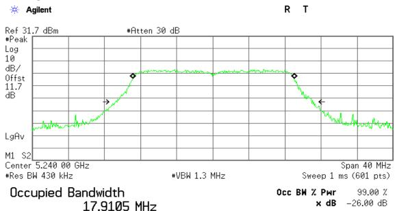
Transmit Freq Error 78.218 kHz x dB Bandwidth 21.866 MHz
