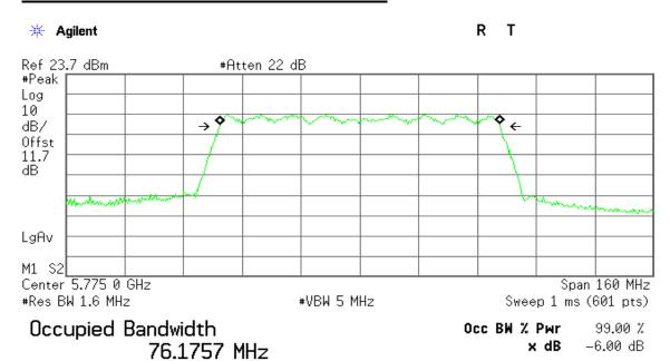
Transmit Freq Error -35.039 kHz x dB Bandwidth 76.596 MHz
