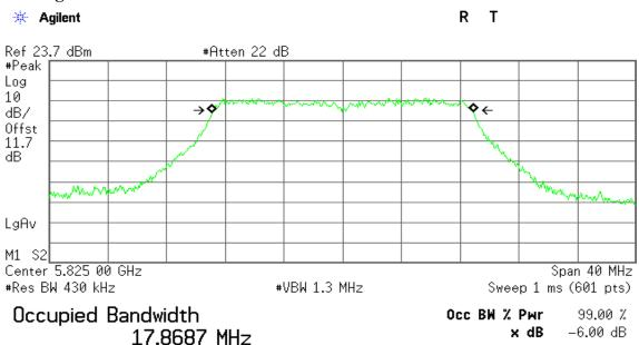
Transmit Freq Error 6.727 kHz x dB Bandwidth 17.671 MHz
