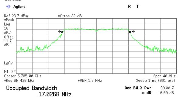
Transmit Freq Error -62.570 kHz x dB Bandwidth 16.501 MHz
