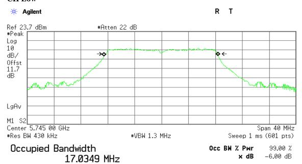
Transmit Freq Error -96.536 kHz x dB Bandwidth 16.586 MHz
