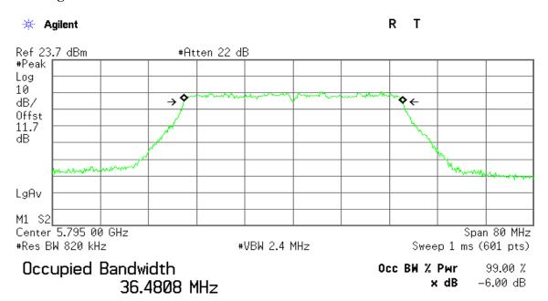
Transmit Freq Error 76.430 kHz x dB Bandwidth 36.329 MHz
