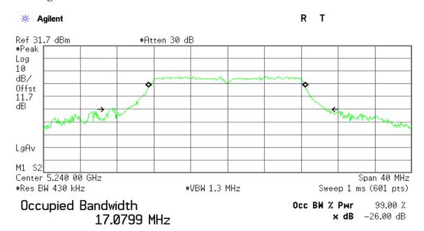
Transmit Freq Error -84.336 kHz x dB Bandwidth 23.432 MHz
