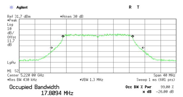
Transmit Freq Error 23.336 kHz x dB Bandwidth 21.391 MHz
