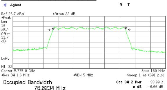
Transmit Freq Error 24.006 kHz x dB Bandwidth 76.322 MHz
