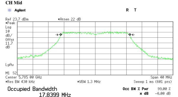
Transmit Freq Error 28.862 kHz x dB Bandwidth 17.654 MHz
