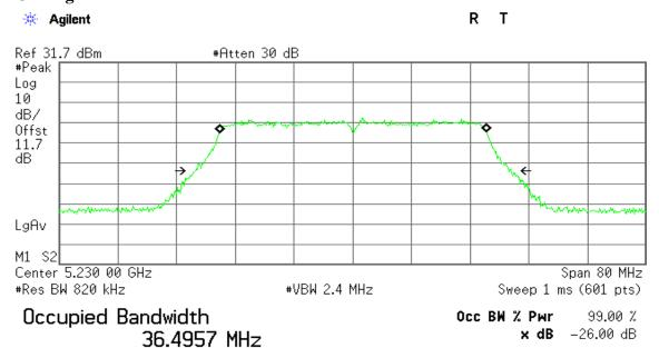
Transmit Freq Error 64.129 kHz x dB Bandwidth 43.078 MHz
