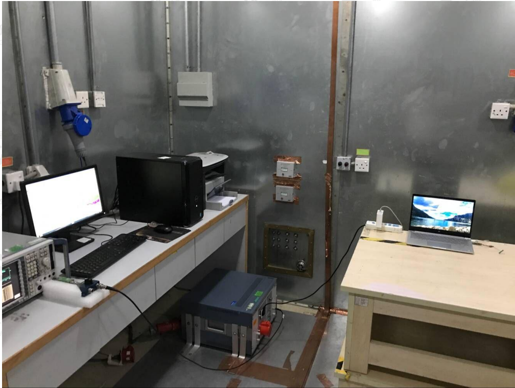
FCC RADIATED EMISSION TEST SETUP BELOW 1GHZ
