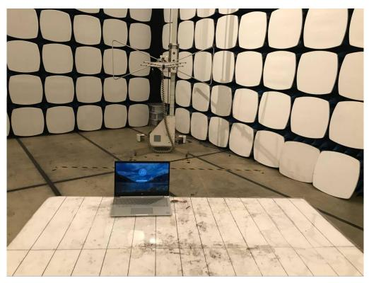
RADIATED EMISSION TEST SETUP ABOVE 1GHZ
