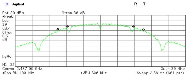
Occupied Bandwidth 15.0636 MHz Occ BW % Pwr 99.00 % x dB -6.00 dB
