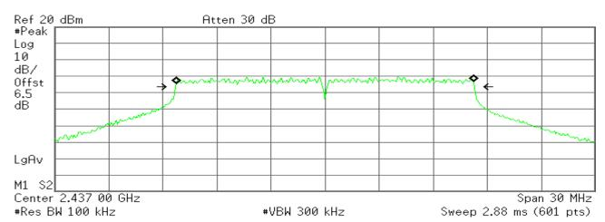
Occupied Bandwidth 16.5075 MHz Occ BW % Pwr 99.00 % x dB -6.00 dB
