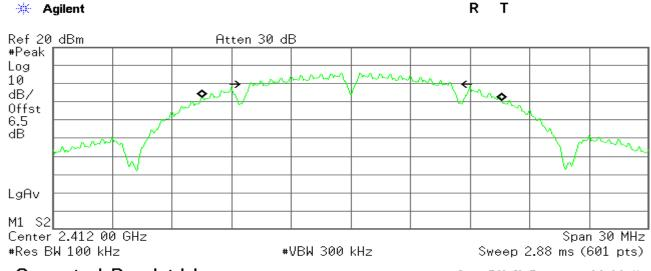
Occupied Bandwidth 15.0988 MHz Occ BW % Pwr 99.00 % × dB -6.00 dB
