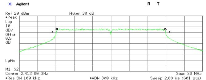
Occupied Bandwidth 17.7243 MHz Occ BW % Pwr 99.00 % x dB -6.00 dB
