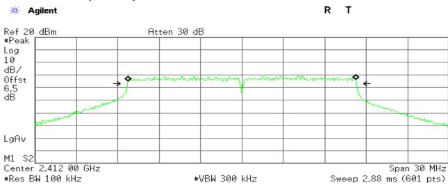
Occupied Bandwidth 16.5142 MHz Occ BW % Pwr 99.00 % x dB -6.00 dB
