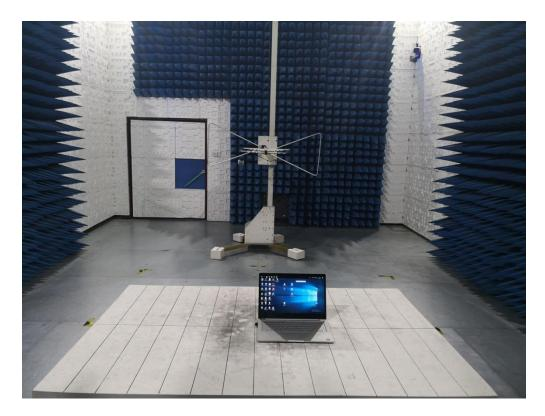
RADIATED EMISSION TEST SETUP ABOVE 1GHZ
