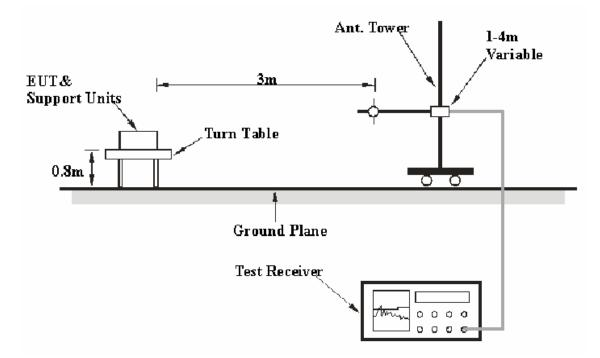
The radiated emission tests were performed in the 3 meters chamber B test site, using the setup accordance with the ANSI C63.4-2003. The specification used was the FCC 15.109, FCC 15.209 and FCC 15.247 limits.
