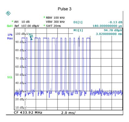
FCC Part15.231 (a) (1) A manually operated transmitter shall employ a switch that will automatically deactivate the transmitter within not more than 5 seconds of being released.
