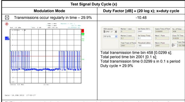
EUT has been operated using the worst-case duty cycle in continuously transmitter mode (regardless normally operated different key function mode).
