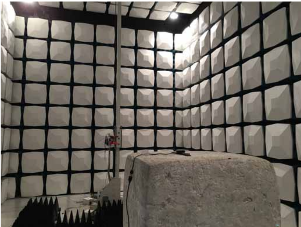
Description: Radiated Emission Test Setup for 1~18GHz
