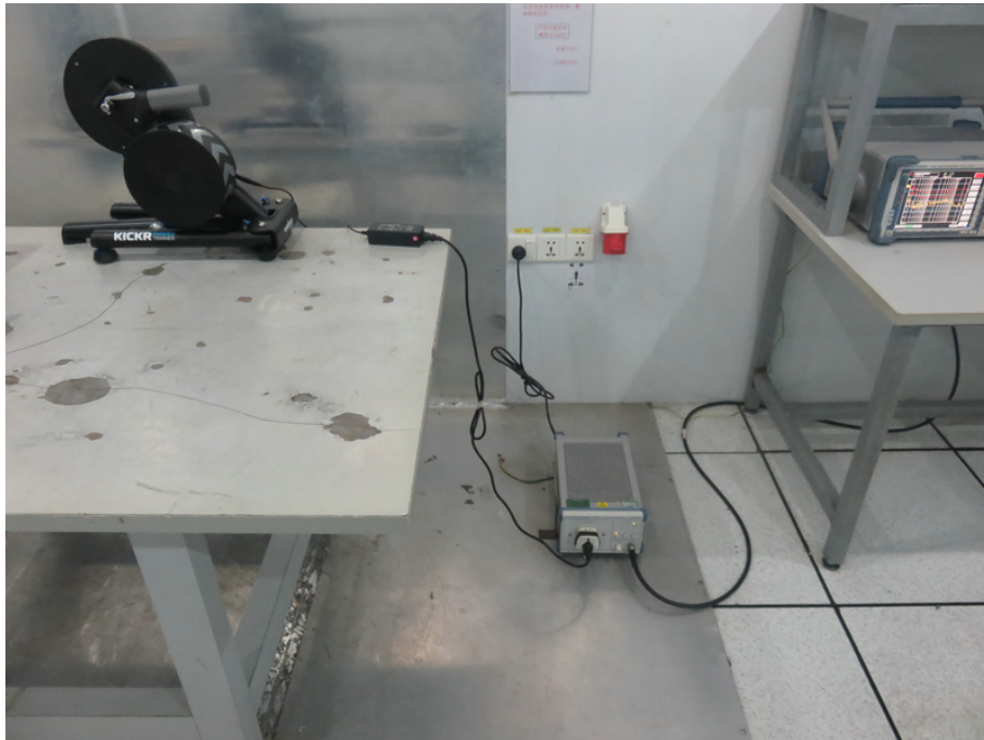
1 Photo of Conducted Emission Test
