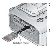
2 Orient the Kodak Wi-Fi<sup>®</sup> card as shown, then push the card into the card slot to seat the connector.
