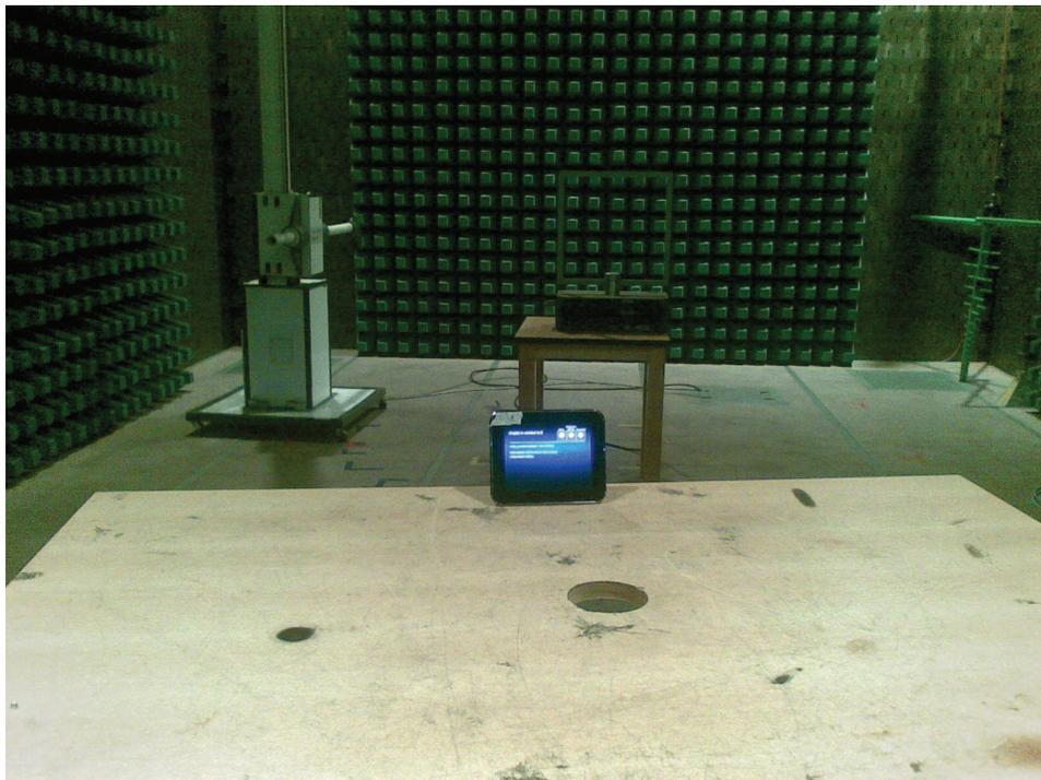
**Photograph 3: Set-up for Radiated Emissions below 1GHz**
