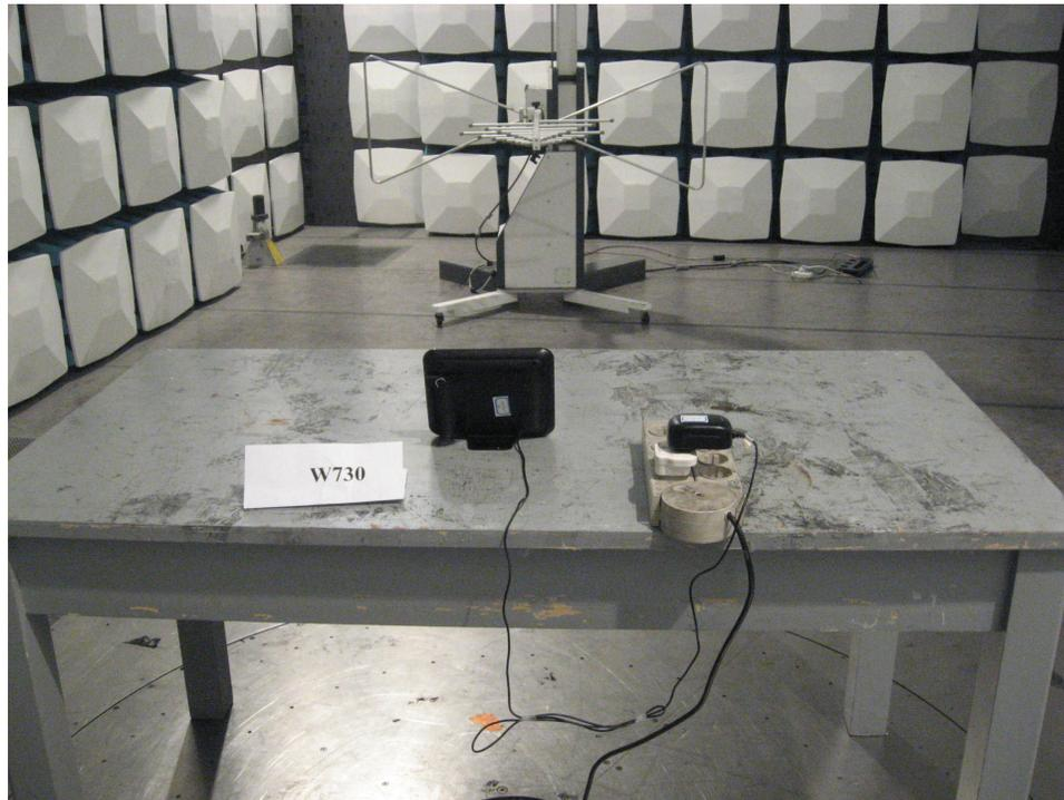
**Photograph 4: Set-up for Radiated Emissions above 1GHz**
