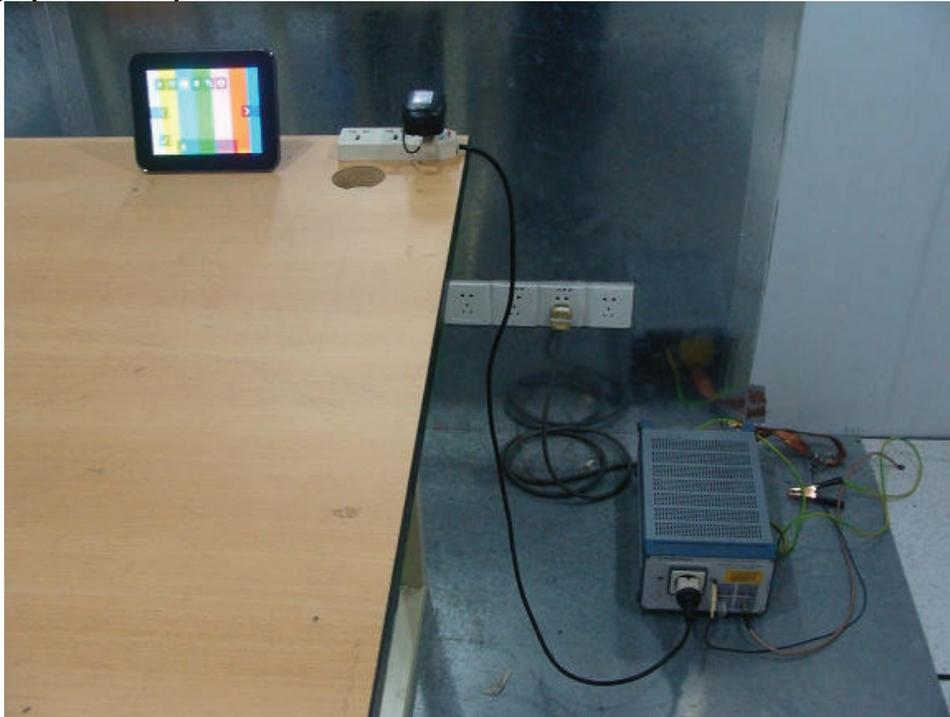
Photograph 2: Set-up for Radiated Emissions below 30MHz
