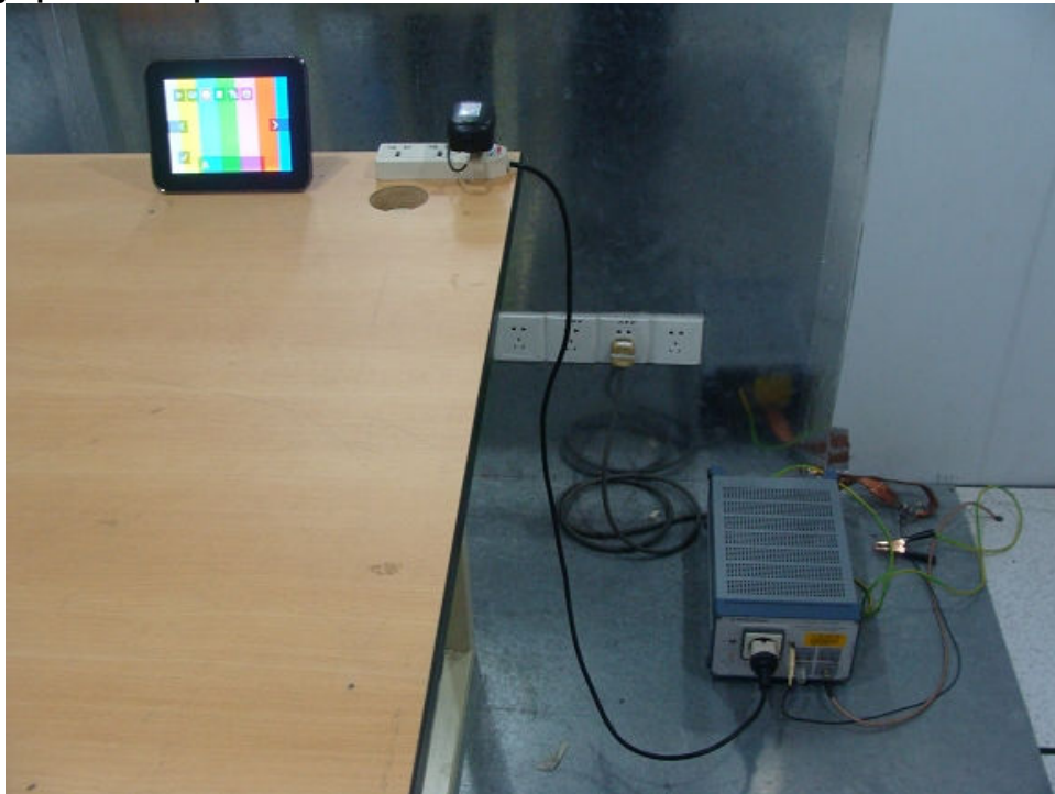
Photograph 2: Set-up for Radiated Emissions below 30MHz
