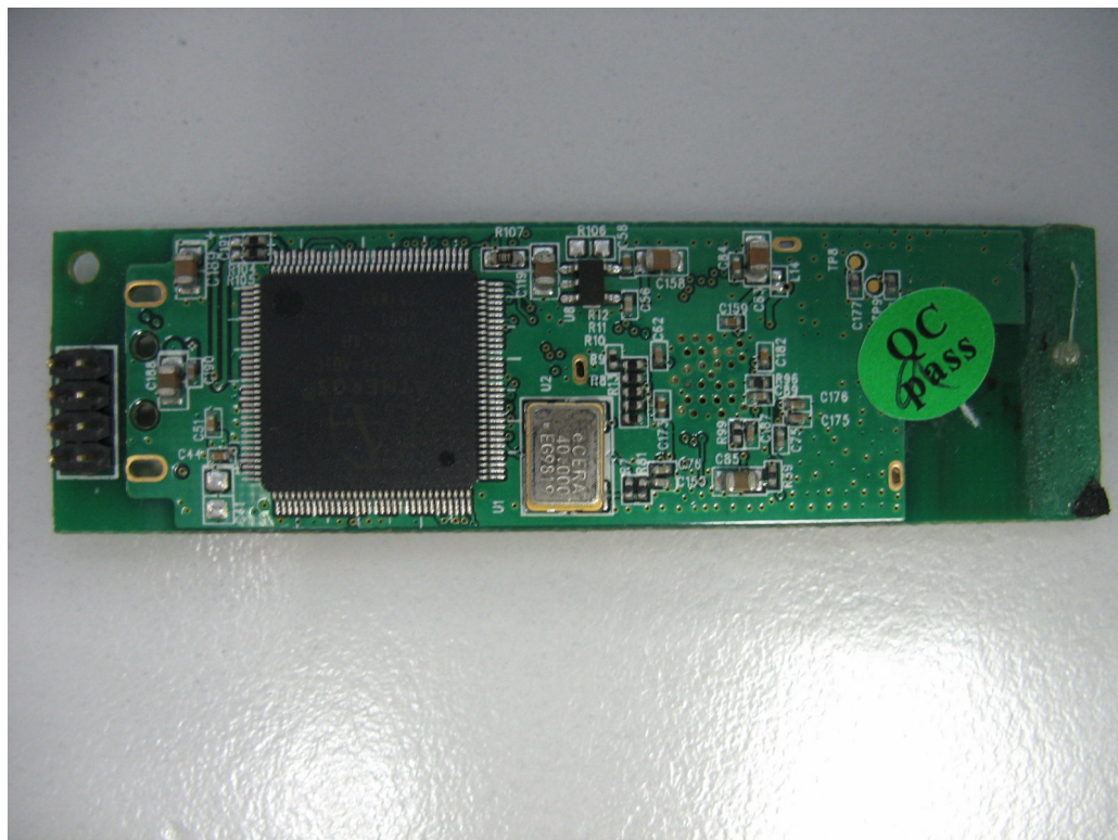
WiFi module PCB (Bottom)
