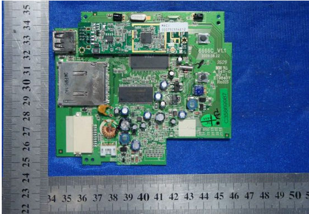
Fig. 5: PCB in photo frame (component side)
