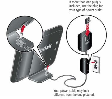
NOTE: The frame automatically turns on when you plug it in for the first time.
