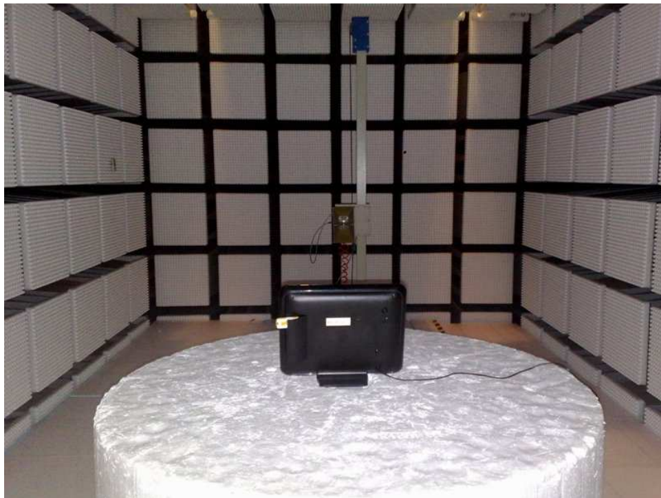
Photograph 4: Set-up for Radiated Emissions above 1GHz
