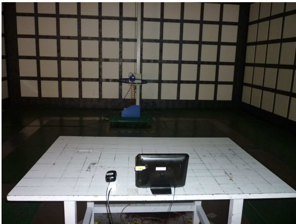
Photograph 2: Set-up for Radiated Emissions below 30MHz
