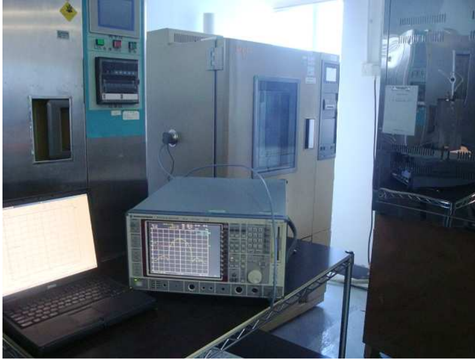
Photograph 5: Setup for Radio Spectrum testing
