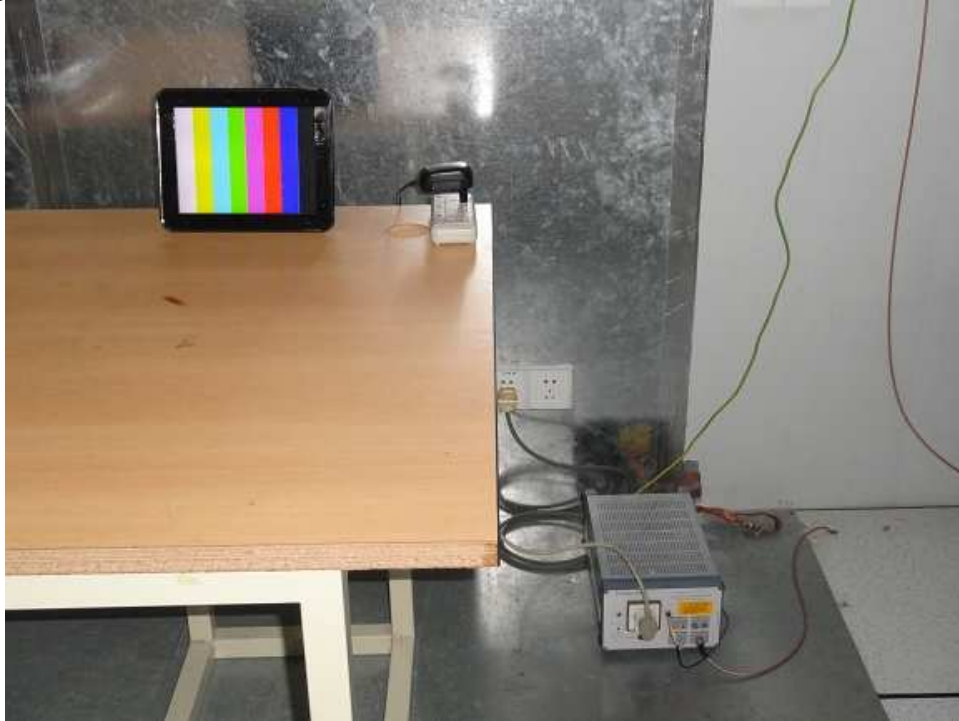
Photograph 2: Set-up for Radiated Emissions below 30MHz
