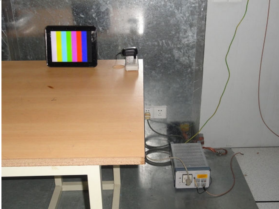
Photograph 2: Set-up for Radiated Emissions below 30MHz
