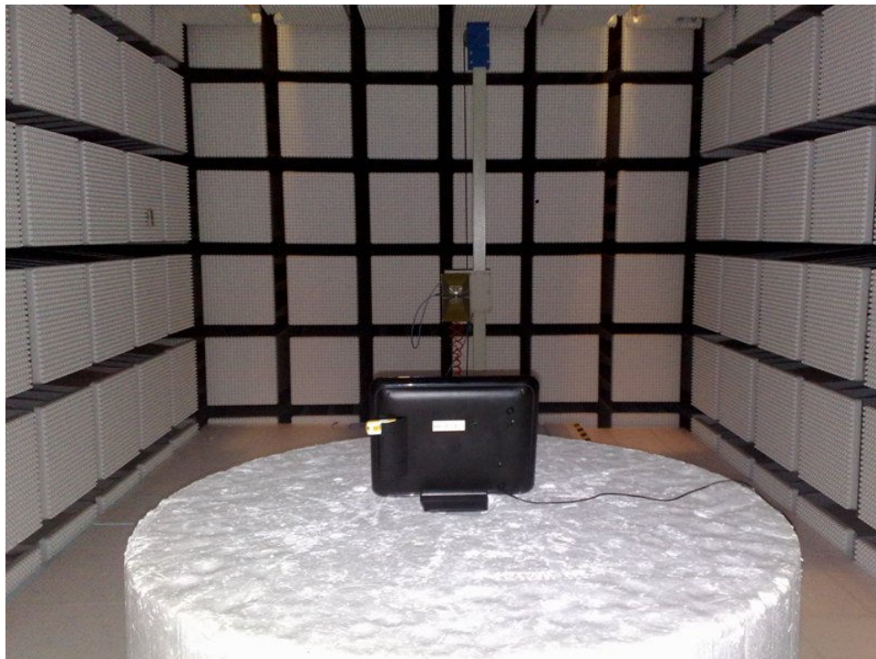
Photograph 4: Set-up for Radiated Emissions above 1GHz
