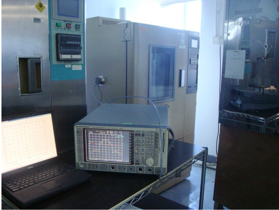
Photograph 5: Setup for Radio Spectrum testing
