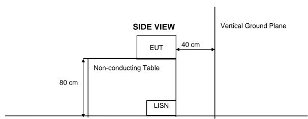
Other Measurements: 2 meters from top of EUT to ceiling 80 cm from closest part of EUT to the LISN
