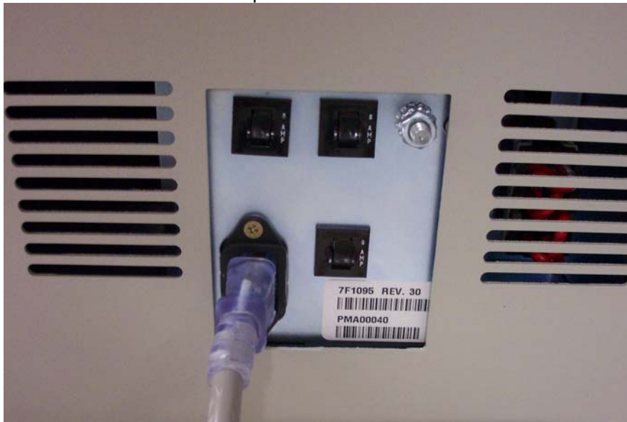
Power Input and Circuit Breakers
