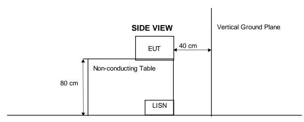
Other Measurements: 2 meters from top of EUT to ceiling 80 cm from closest part of EUT to the LISN
