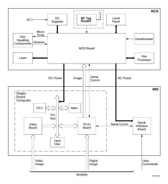
Note: Broken line block identifies new intentional radiator RF subsystem being added to printer.
