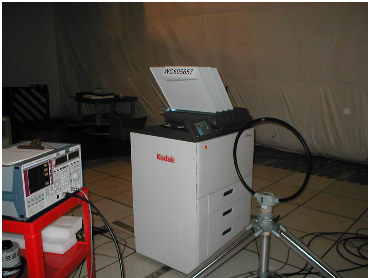
Test-setup photo(s): General Field Strength Limits 0.009 – 30 MHz
