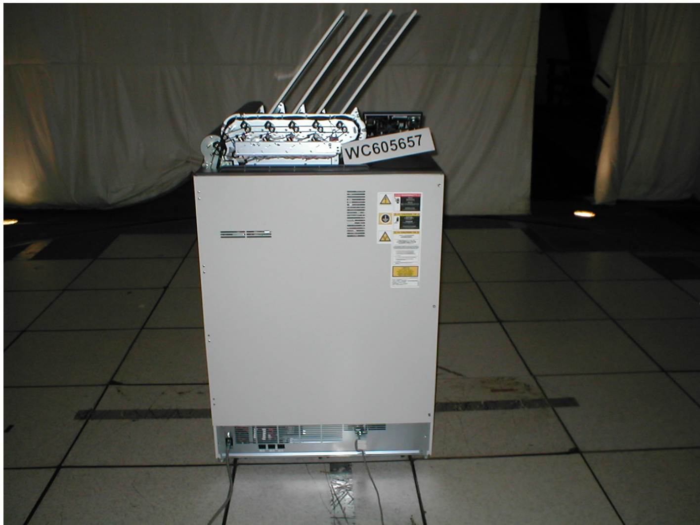
Test-setup photo(s): Radiated Emissions 30 - 1000 MHz
