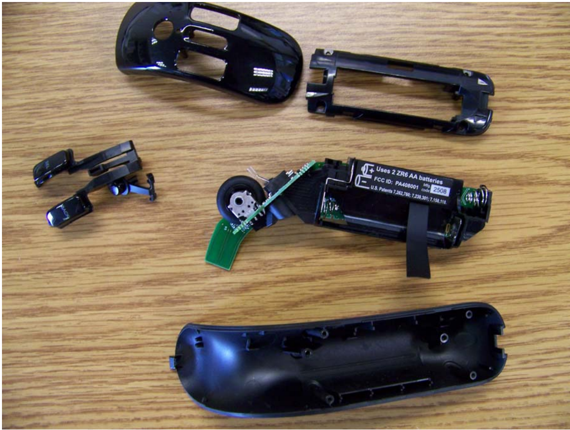
Kodak remote PCB with 2.4 GHz radio and sensor PCB identified
