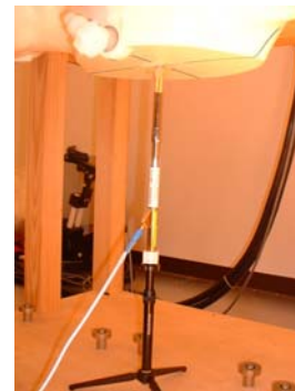
2450MHz System performance check setup
