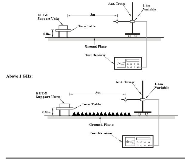
The radiated emission tests were performed in the 3 meters, using the setup accordance with the ANSI C63.4-2009. The specification used was the FCC 15.209 and FCC 15.247 limits.
