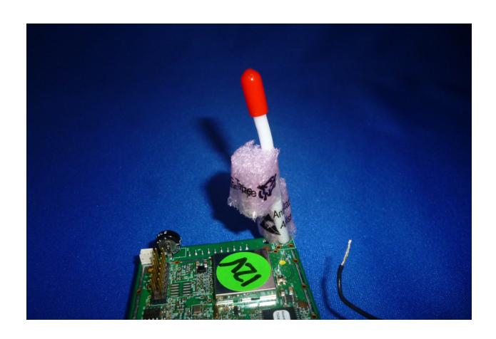
On board Through-hole Wire antenna, 0.0dBi Gain
