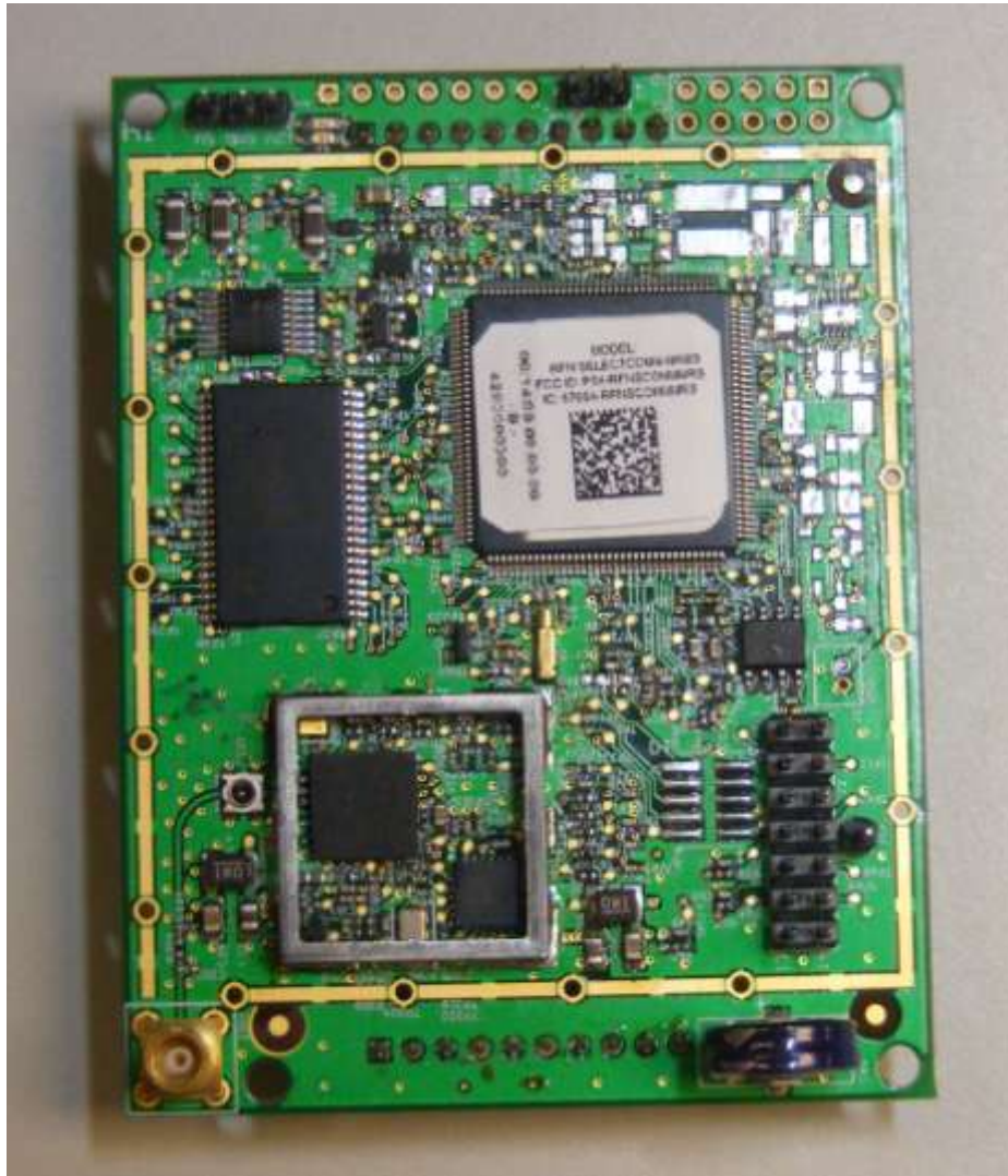
Figure 3: RFN SelectComm-MRB3 – Top, shields removed
