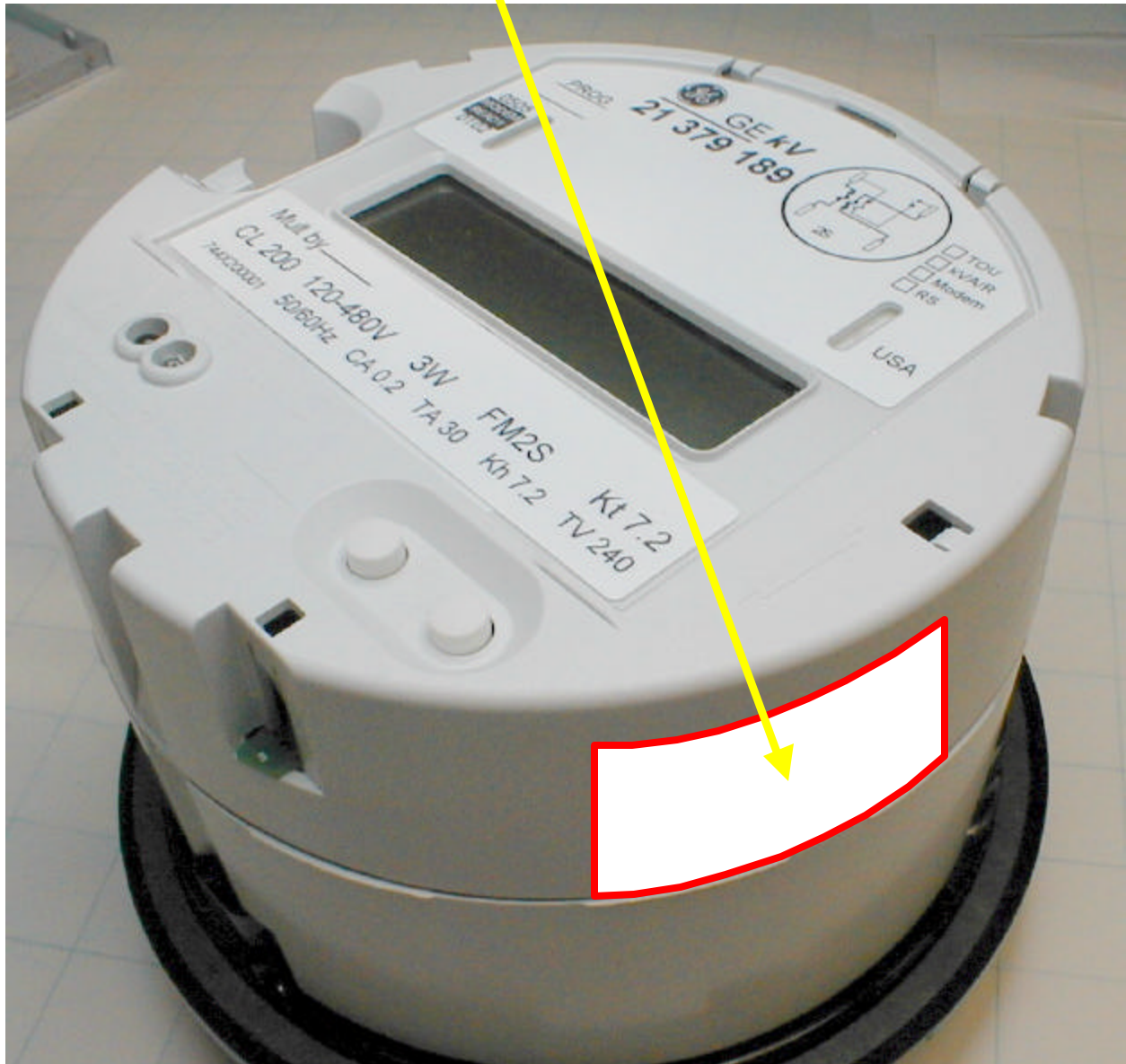
FCC Label Location, Electric Service Meter (GE)
