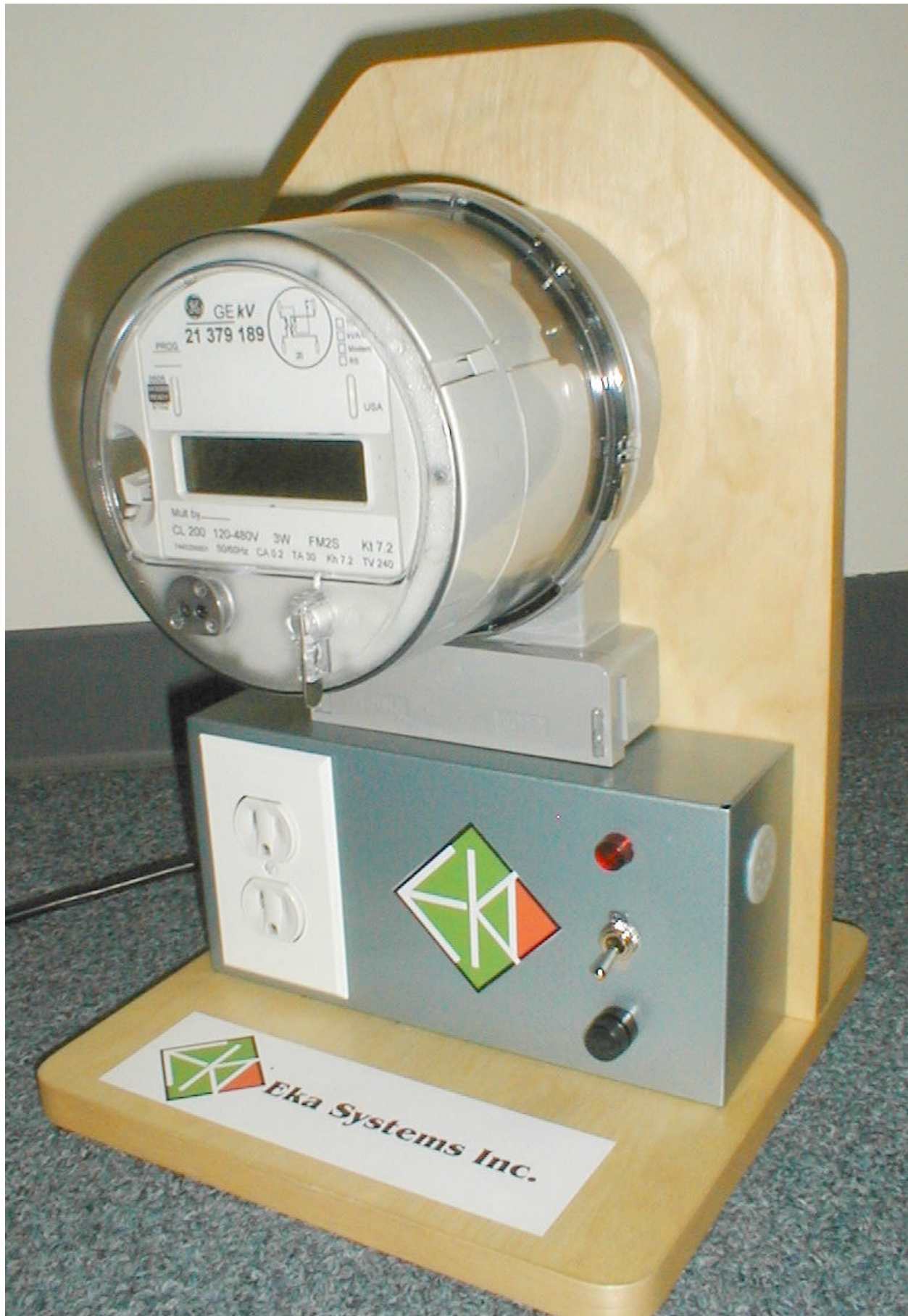
Electric Service Meter (GE) Test Fixture
