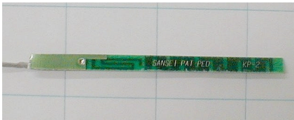
Internal Antenna Board, Front
