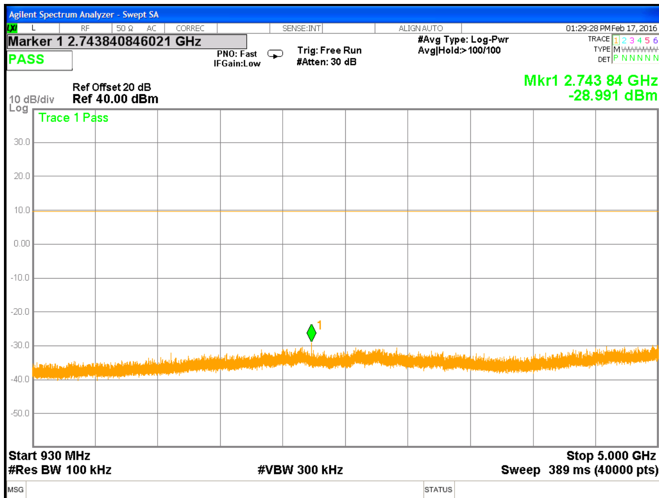
Figure 21: Conducted Spurious Emissions, High Power, Center Channel 930-5000MHz
