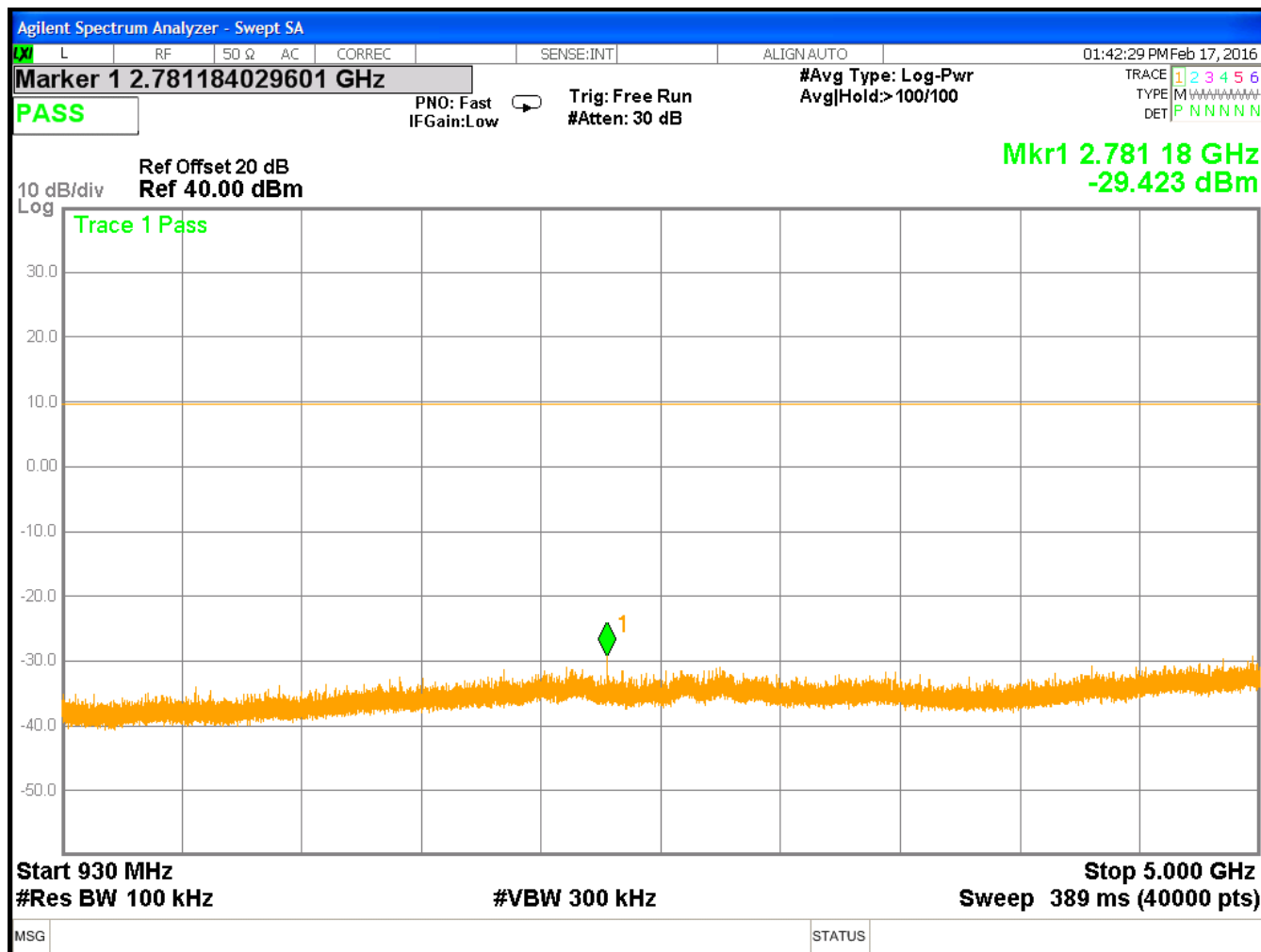
Figure 37: Conducted Spurious Emissions, Low Power, High Channel 930-5000MHz
