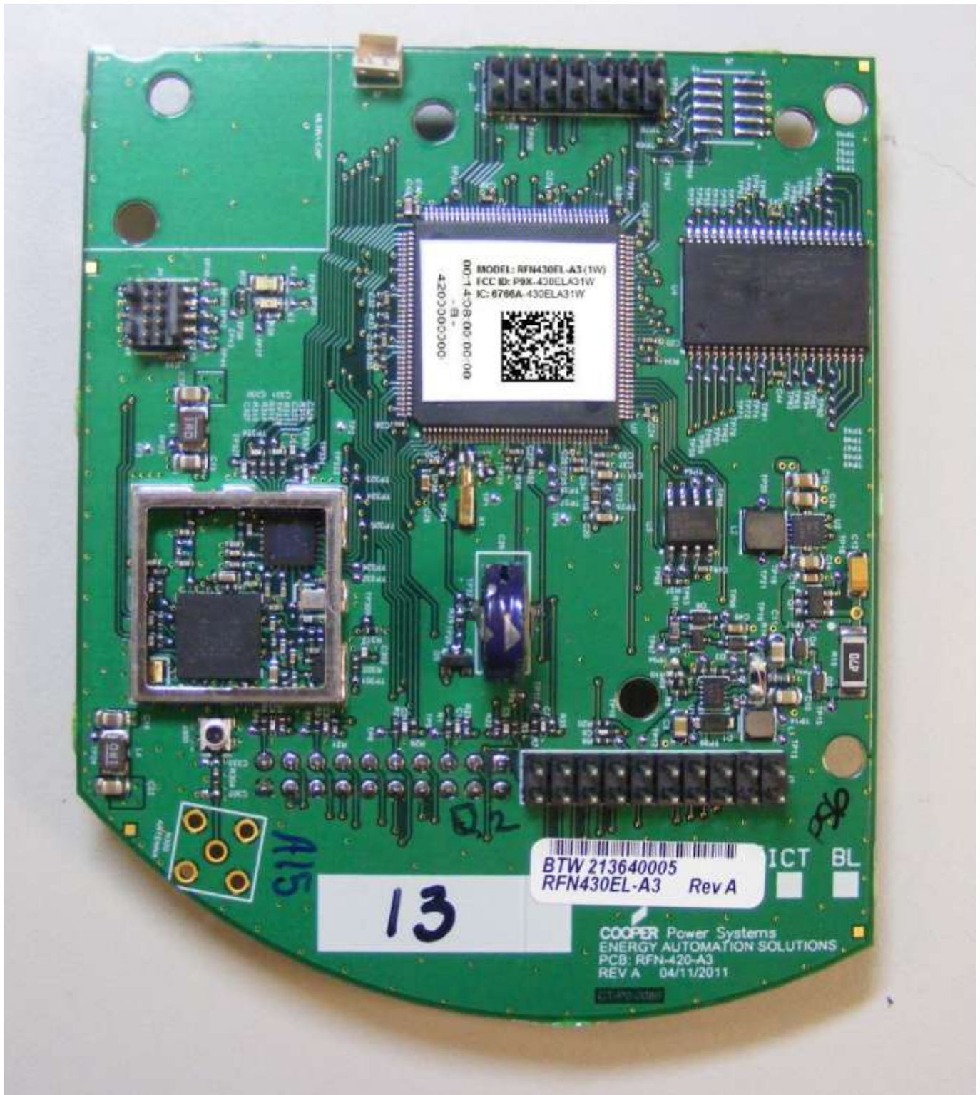
Figure 3: RFN430EL-A3 (1W) – Top, shields removed
