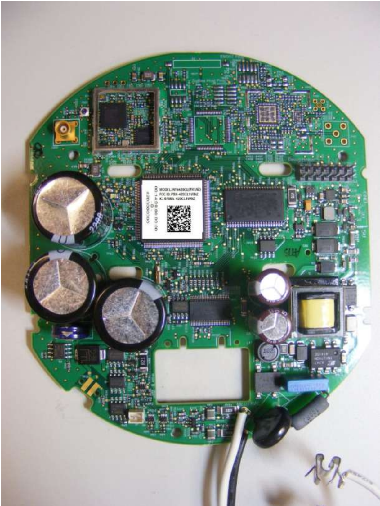
Figure 3: RFN420CL (1W,NZ) – Top, shields removed
