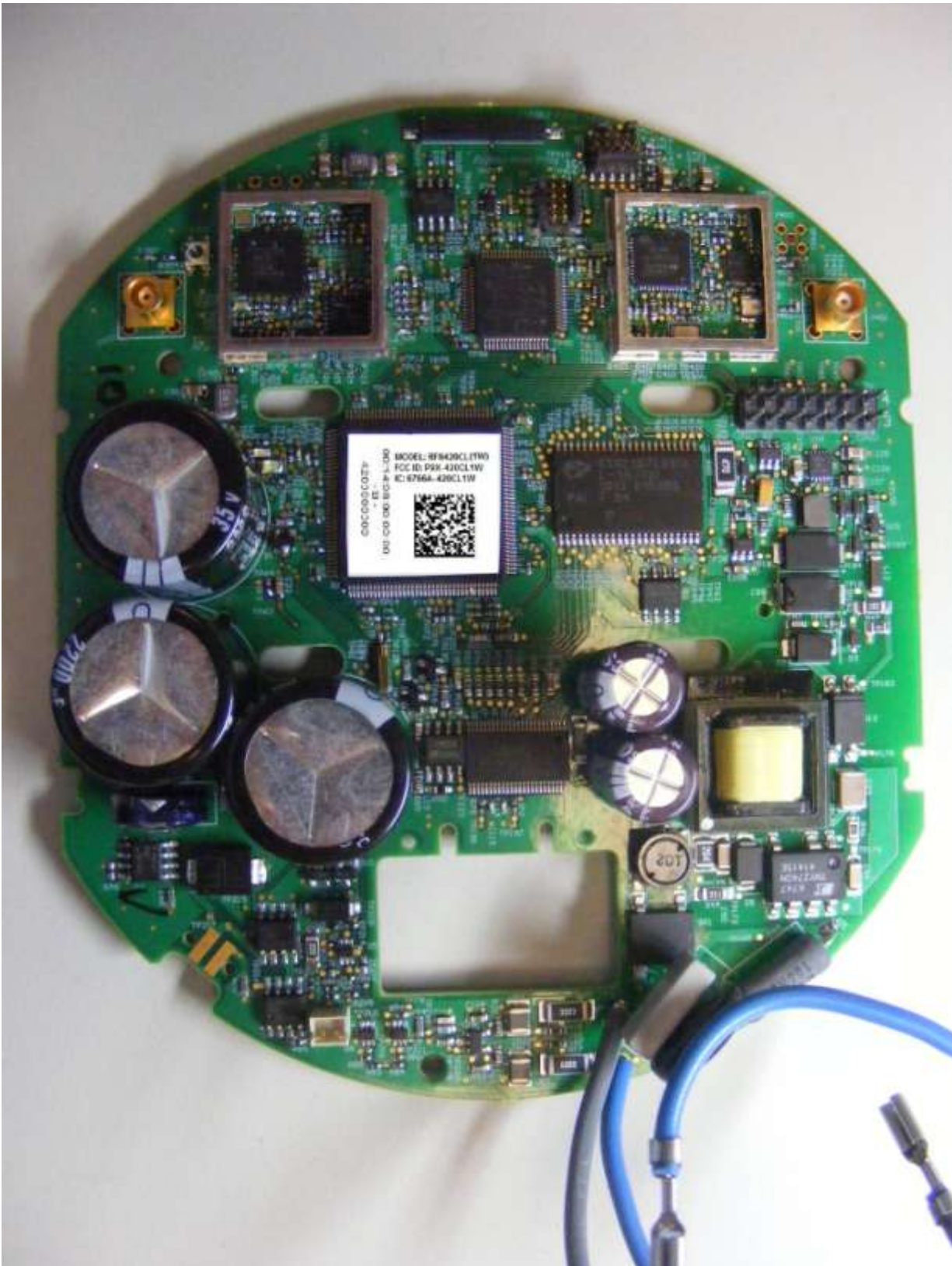
Figure 3: RFN420CL (1W) – Top, shields removed
