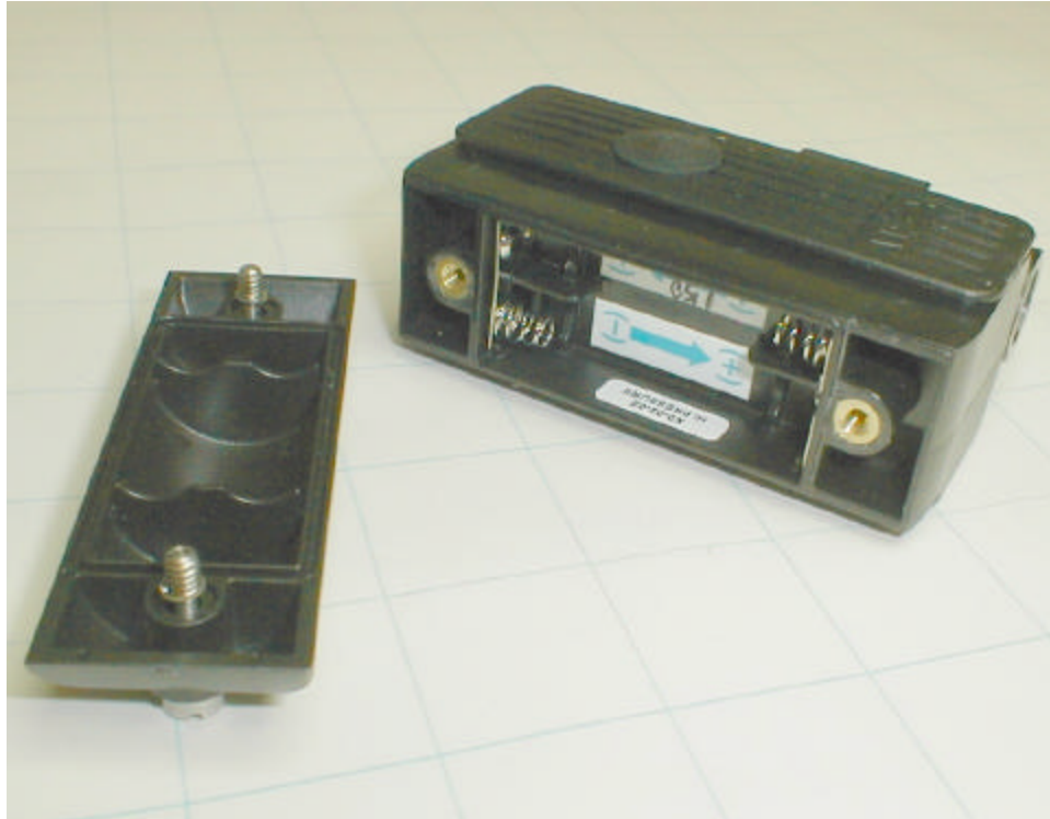
Battery Cover Removed
