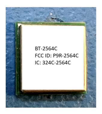
The label is a matt-white uncoated paper with a general purpose permanent, acrylic based pressure sensitive adhesive. It is affixed to the top of the shielding.
