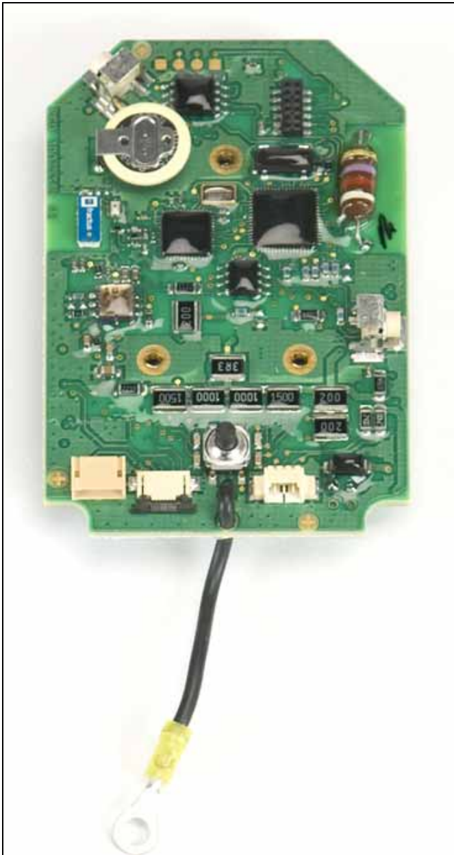
Control board - Front
