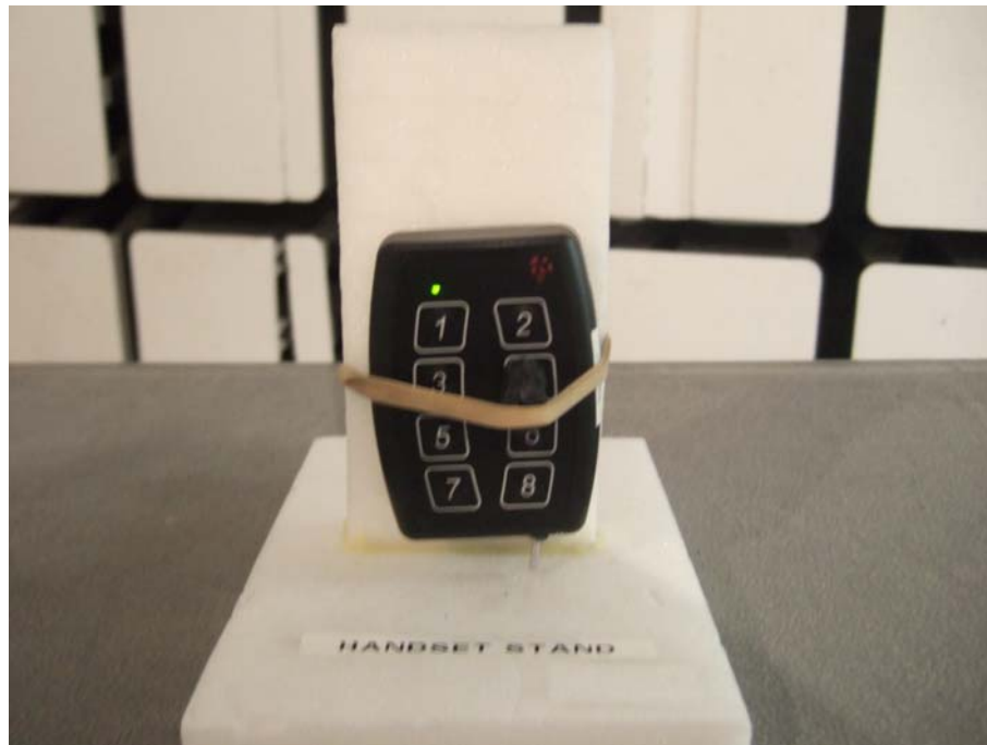
Radiated Emissions (Enclosure Port) Test Setup
