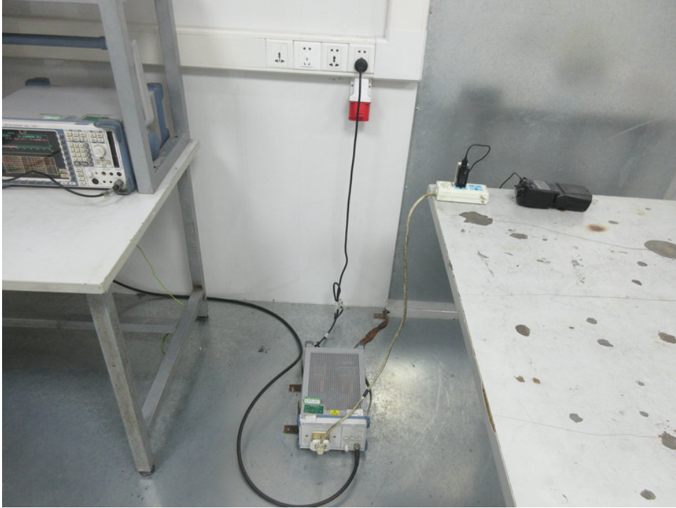
Photo of Conducted Emission Test
