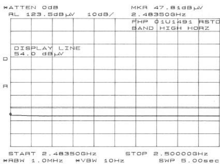
**12 dBi PATCH ANTENNA - SPURIOUS RADIATED EMISSIONS**
