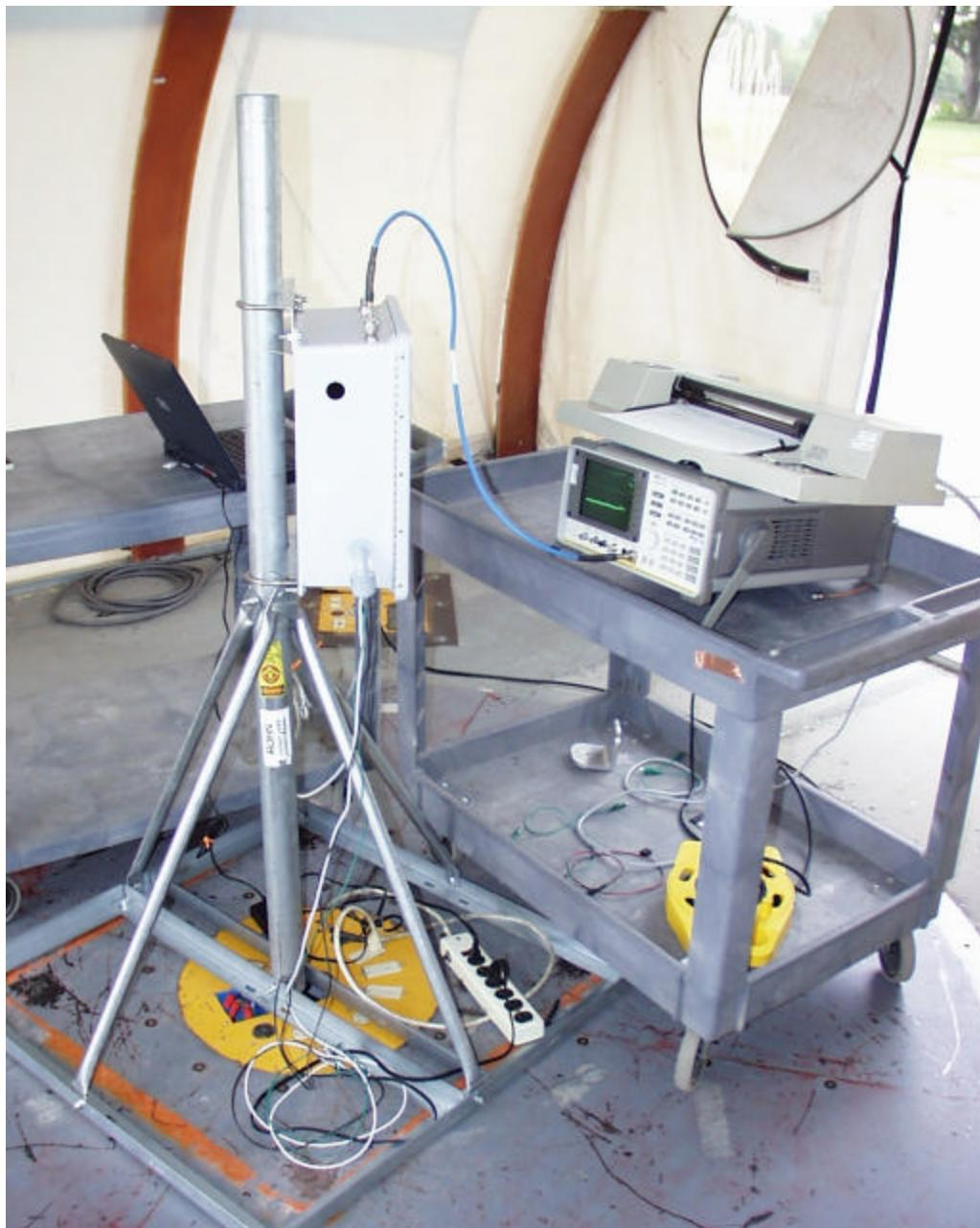
**TRANSMITTER RADIATED RF MEASUREMENT SETUP FOR 15.0 dBi OMNI ANTENNA**
