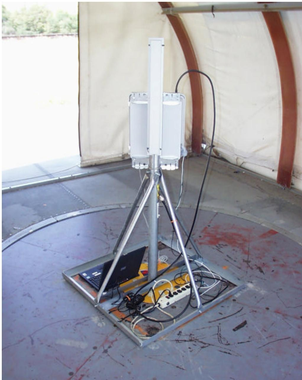
**TRANSMITTER RADIATED RF MEASUREMENT SETUP FOR 7.4 dBi OMNI ANTENNAS WITH RECEIVE DIVERSITY**
