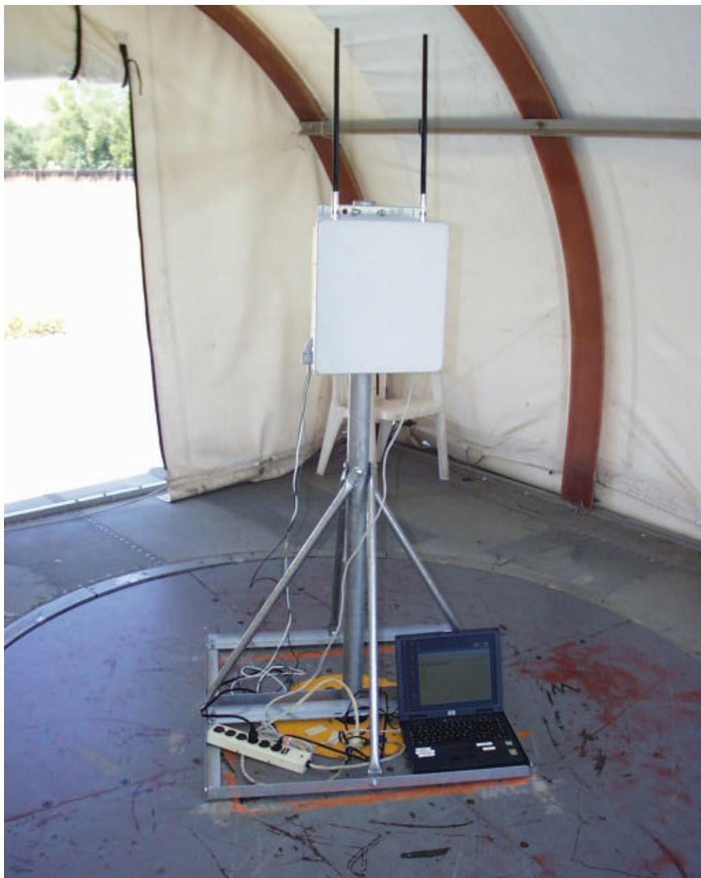
**TRANSMITTER RADIATED RF MEASUREMENT SETUP FOR 7.0 dBi OMNI ANTENNAS WITH COUNTERPOISE GROUND PLANE AND RECEIVE DIVERSITY**
