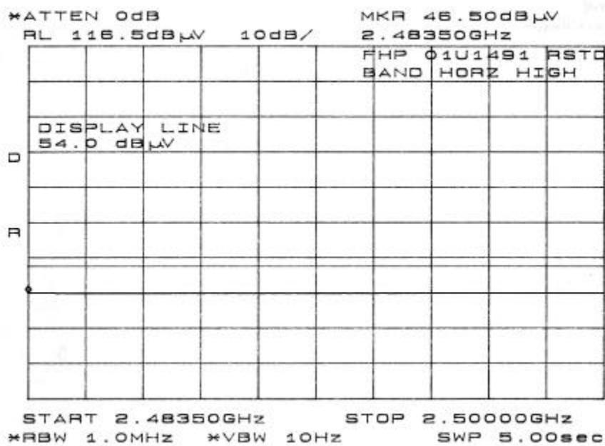
**7.4 dBi OMNI ANTENNAS - SPURIOUS RADIATED EMISSIONS**
