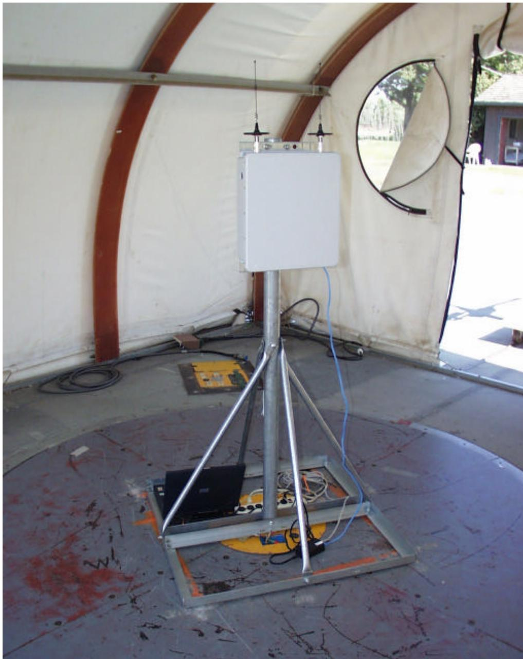
**POWERLINE CONDUCTED EMISSIONS MEASUREMENT SETUP FOR SELF-CONTAINED POWER**
