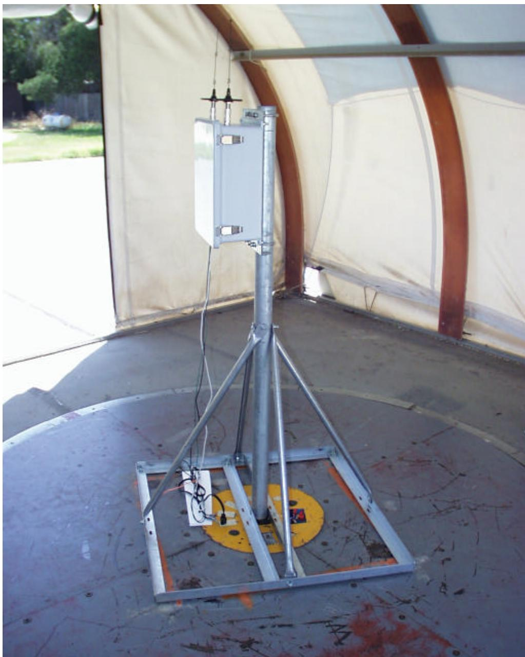
**DIGITAL DEVICE RADIATED EMISSIONS MEASUREMENT SETUP FOR POWER OVER ETHERNET**
