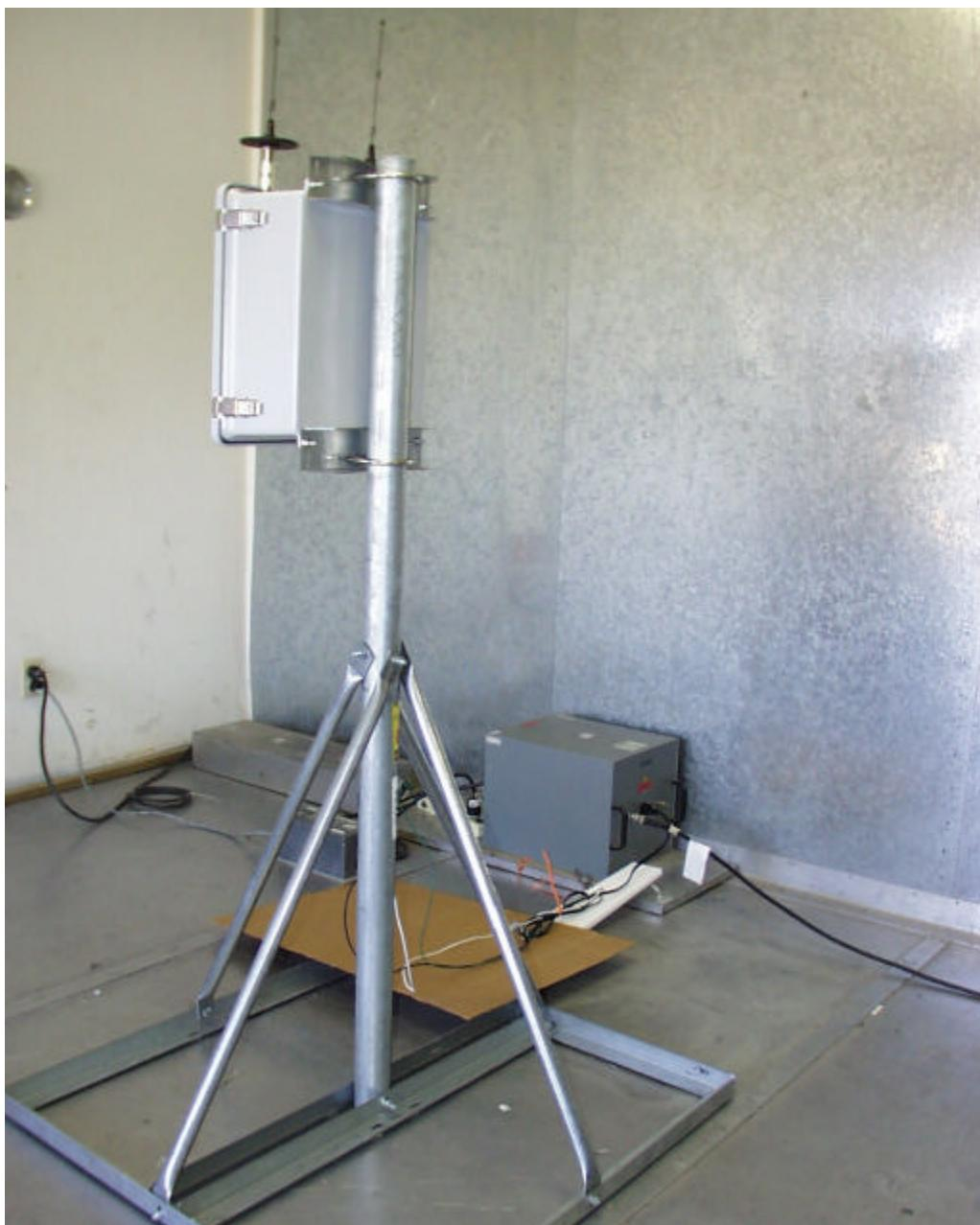
**POWERLINE CONDUCTED EMISSIONS MEASUREMENT SETUP FOR POWER OVER ETHERNET**
