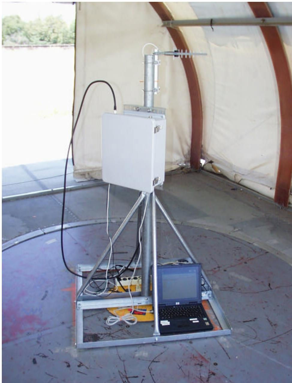
**TRANSMITTER RADIATED RF MEASUREMENT SETUP FOR 12.0 dBi PATCH ANTENNA**
